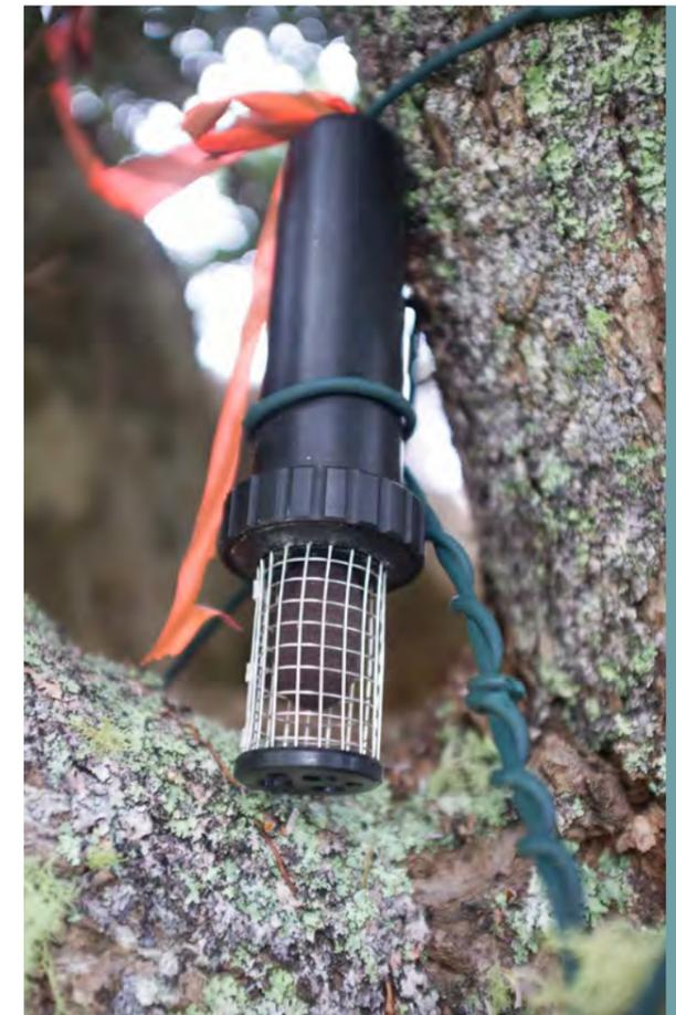
An acoustic recorder used to detect seabird calls.
